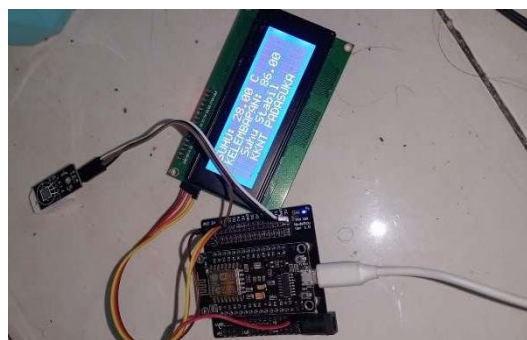
Figure 4. Active Control and Sensor System
