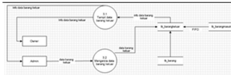
Figure 16. Data Flow Diagram Level 2 Process 3.0
