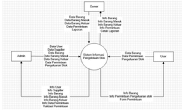
Figure 12. Data Flow Diagram Level 0
