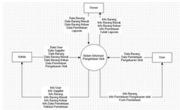
Figure 12. Data Flow Diagram Level 0
