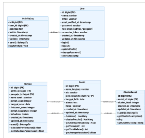
Figure 6. Class Diagram Design
